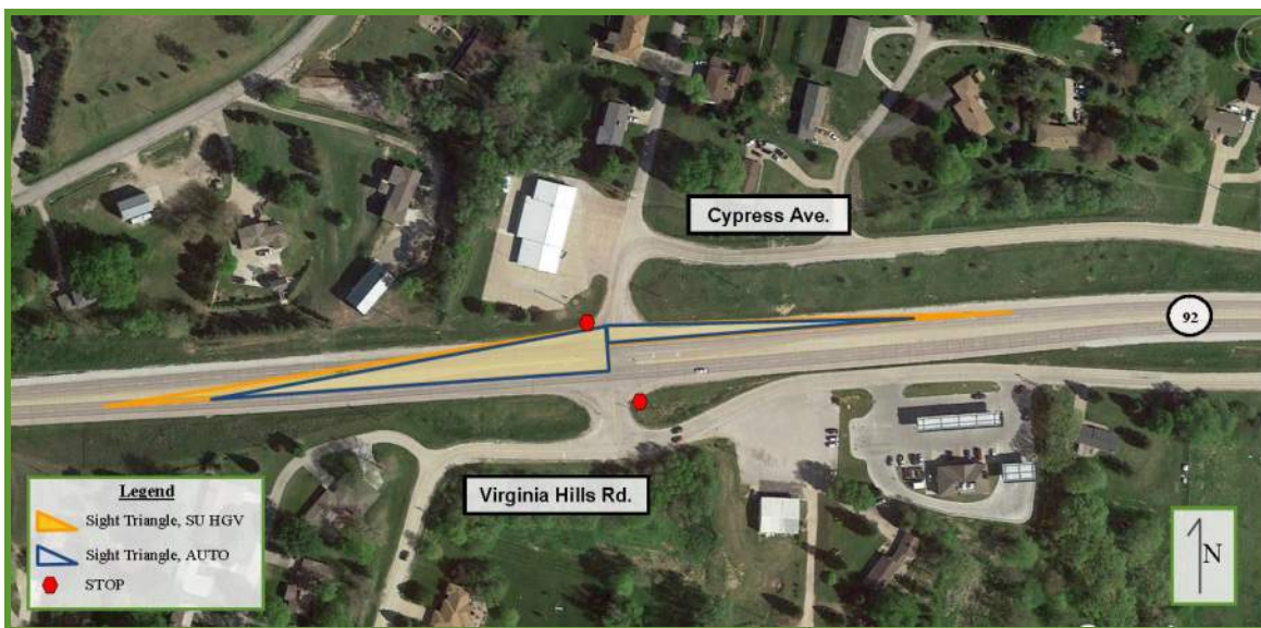
Exhibit 7 – Required Sight Distance Triangles for SB Vehicles
