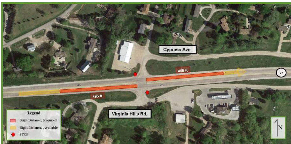
Exhibit 6 – Required Stopping Sight Distance
