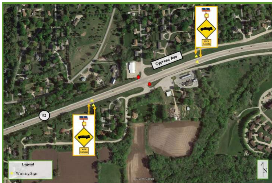
Exhibit 11 – Activated Flashing Warning Beacon System
