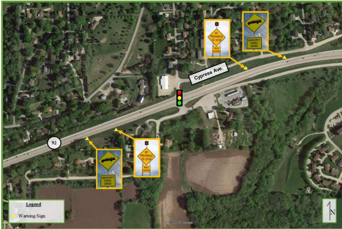
Exhibit 12 – Advanced Warning Sign Locations along Iowa Highway 92
