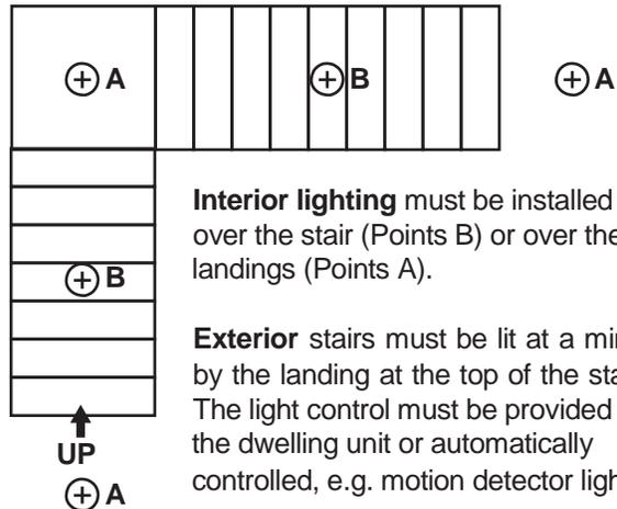
**Interior lighting** must be installed either over the stair (Points B) or over the landings (Points A).
